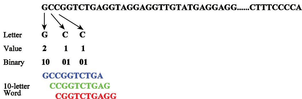
Figure 1. Application of the DNA monkey test to biological sequence analysis. The DNA test counts 10-letter missing words from a 4-letter alphabet (A, C, G, T/U). Three overlapping 10-letter words are shown in blue, green, and red, respectively.
